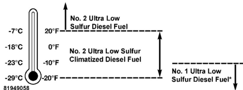
\*No. 1 Ultra Low Sulfur Diesel Fuel (ULSD) should only be used where extended arctic conditions (-10°F/-23°C) exist.
