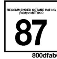
All engines (except 5.7L engines) are designed to meet all emissions regulations and provide excellent fuel economy and performance when using high-quality unleaded “regular” gasoline having an octane rating of 87. The use of premium gasoline is not recommended, as it will not provide any benefit over regular gasoline in these engines.
